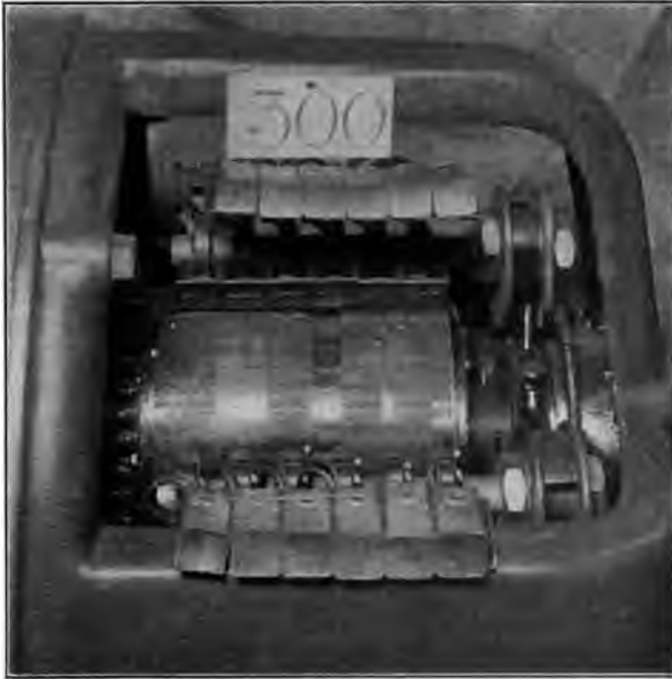
FIG. 86.—Scored commutator surface resulting from the brushes sticking in the holders and selective commutation. Note smooth bands where good commutation was observed.
